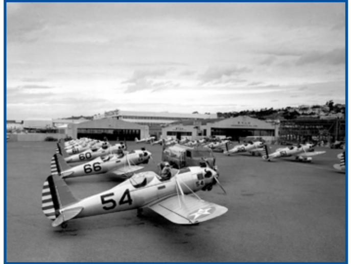
The PT-20As at the Ryan Co. at Lindbergh Field. Mine isn't in view in this picture but I'm sure it was there. It had a field number 57. In 1939, only 30 PT-20 were manufactured. All but one was re-engined with a 125 hp Kinner engine.
